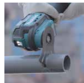
Cutting PVC, FRP pipes
