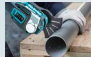
Cutting PVC, FRP pipes
