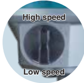
Mechanical 2-speed gearing
