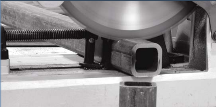
Carbide-Tipped Blades make Virtually Spark-Free Cuts
